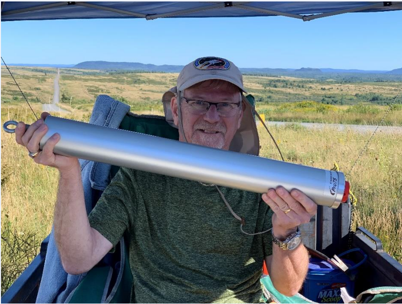
Figure 13 - Look at the size of a CTI 75mm M motor that Bill Daigle is going to use for his Level 4 certification flight!
