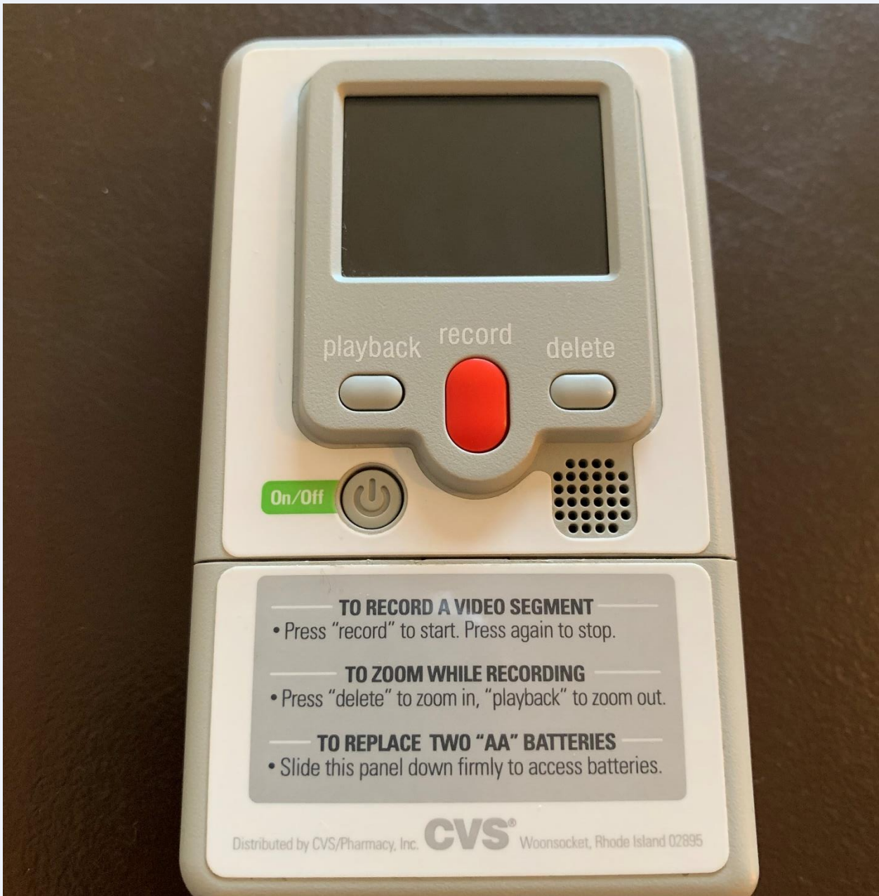
Figure 4 The backside of the CVS Camcorder shows the many features including a playback screen.
