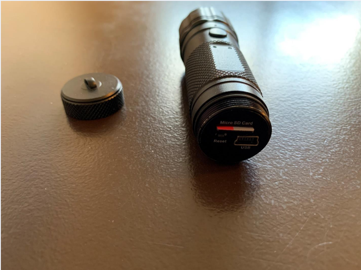
Figure 8 The GearCam has a water-resistant case and can take up to a 16Gb micro SDHC card.
