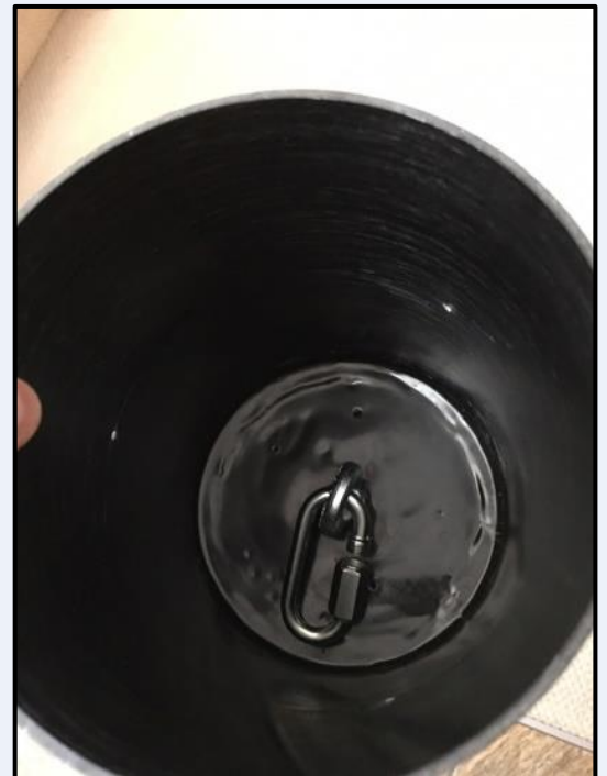
into aluminum nose tip and attached to steel eye nut in photo.
