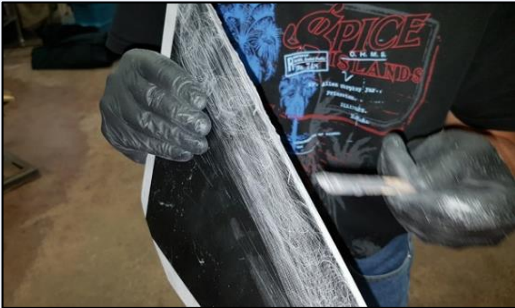
Fin roots buttered with JB Weld.
