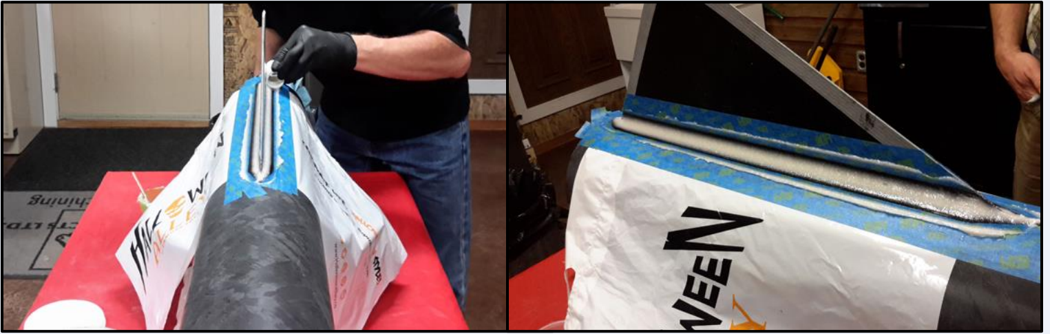
Making external fillets with West System epoxy and Colloidal Silica as a filler to the consistency of peanut butter.
