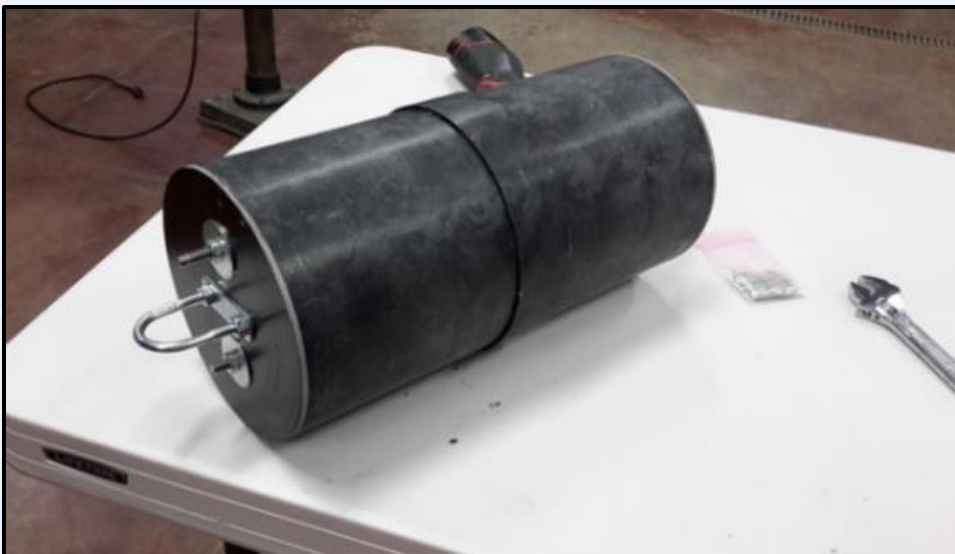
Nose cone bulk plate epoxied into nose cone coupler. 1/4" all thread
