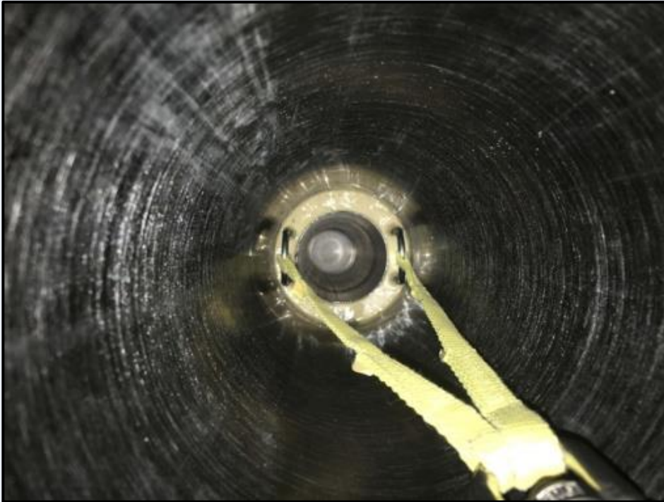
Nose cone bulk plate epoxied into nose cone coupler. 1/4" all thread
