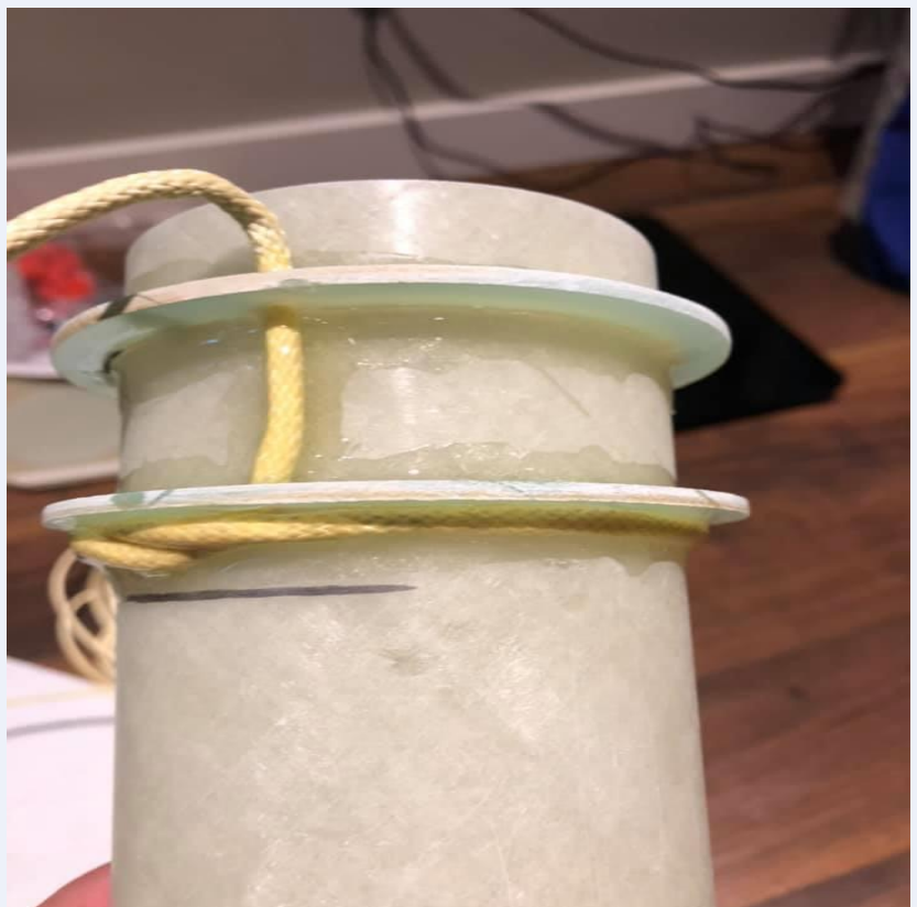
Motor Mount upper centering rings with lower recovery harness attached.
