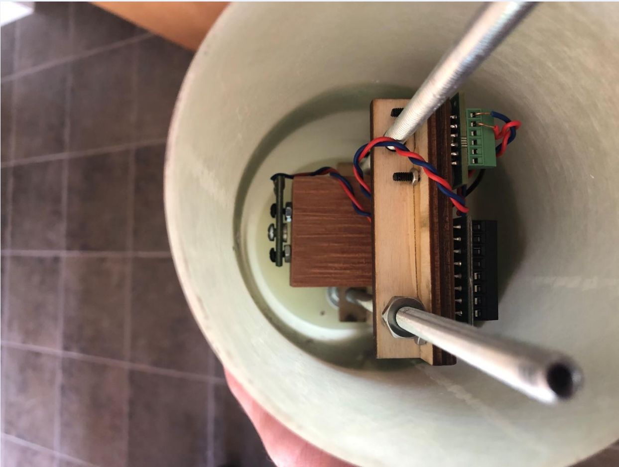
Final E-bay Sled Layout with Switch.
