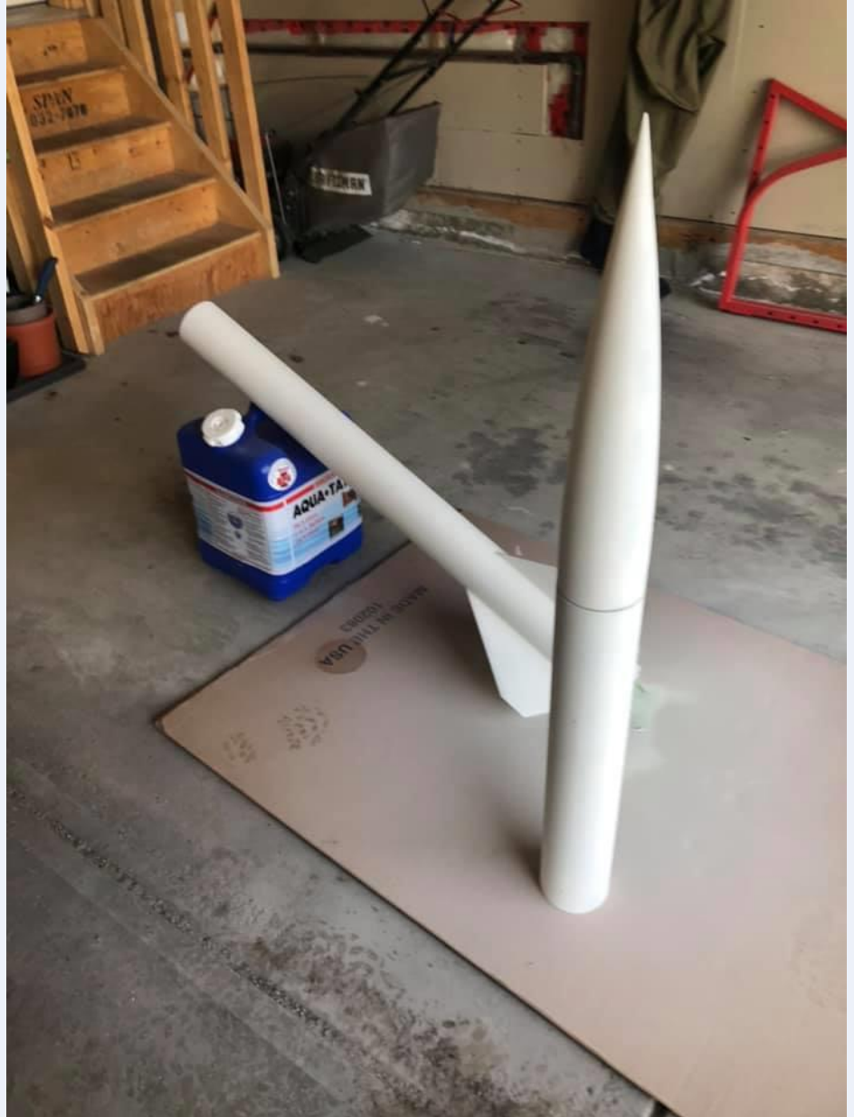
Airframe with KILZ primer applied post sanding.
