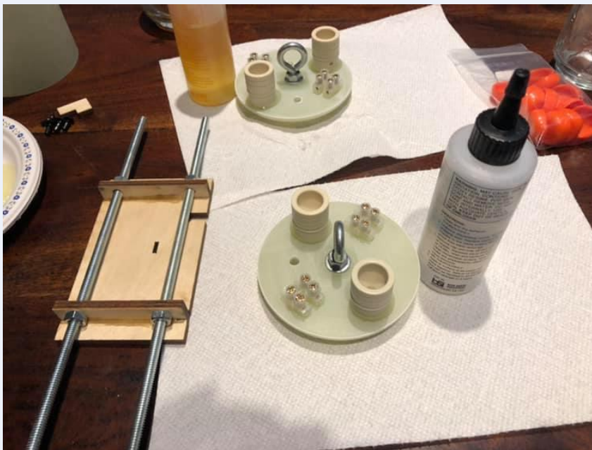
Mounting PVC Ejection Charge Holders and Terminal Blocks onto the Bulkheads
