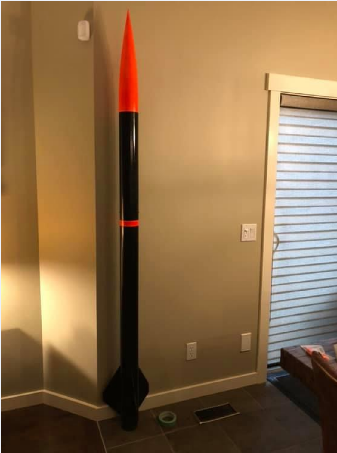
Final Paint Scheme, and First Assembly post finishing. Final weight with Motor 10.3 KG
