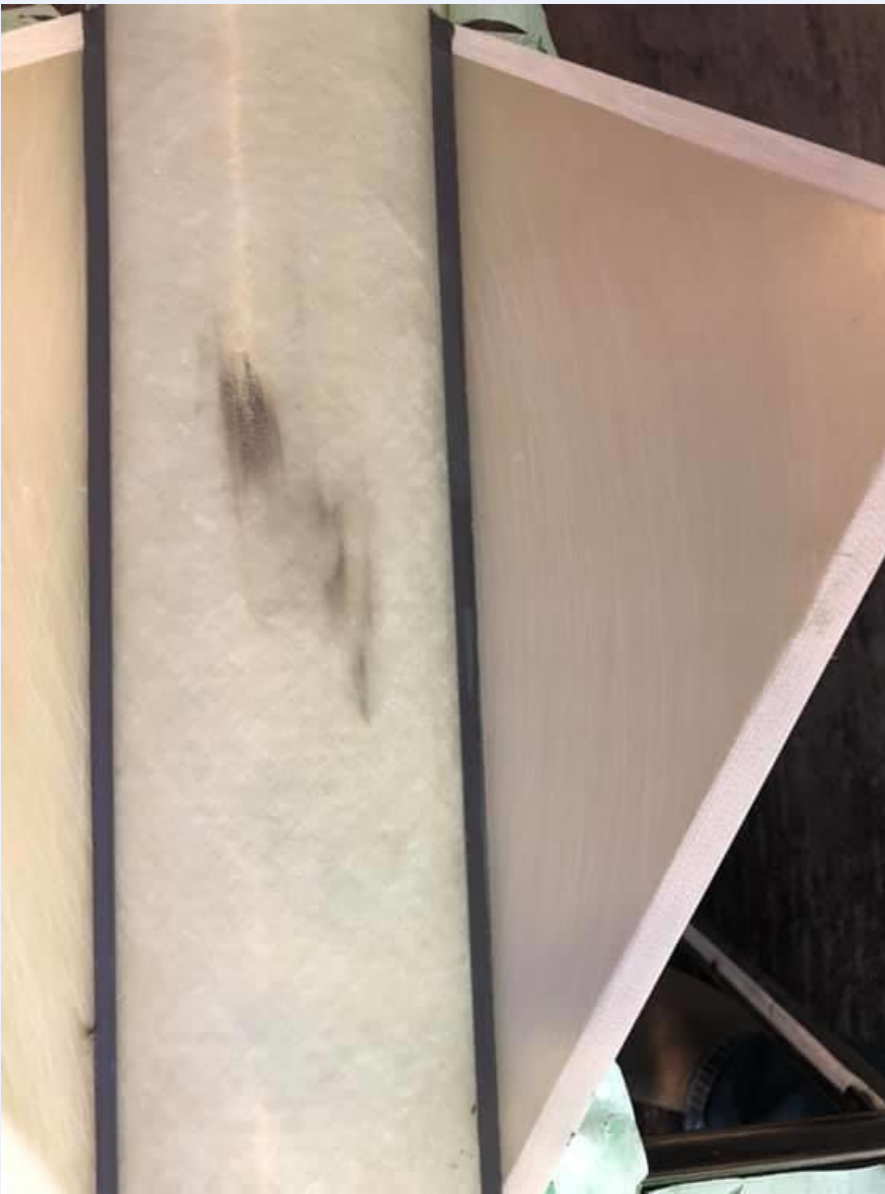
Fin Fillets done with JB Weld and a Large Tongue Depressor
